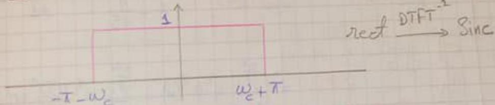
$$h(n) = \text{DTFT}^{-1}[H(\omega)] = \frac{1}{2\pi} \int_{-\pi}^{\pi} H(\omega) e^{j\omega n} d\omega$$
