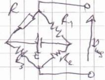
\*  $\theta = 0^\circ\text{C} \Rightarrow R = R_0 = 80 \Omega$  et  $U_{me} = 0 \Rightarrow R_0 R_2 - R_1 R_3 = 0$
