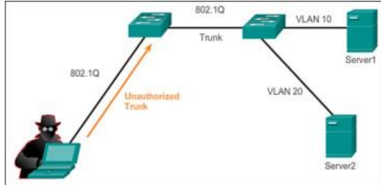
**Protection:** Turning off trunking on all ports, except the ones that specifically require trunking. On the required trunking ports, disable DTP and manually enable trunking.
