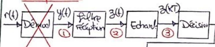
$$\begin{aligned} \textcircled{1} \Rightarrow y(t) &= r(t) \\ y(t) &= u(t) + b(t) \\ &= a(t) * h_e(t) + b(t) \end{aligned}$$
