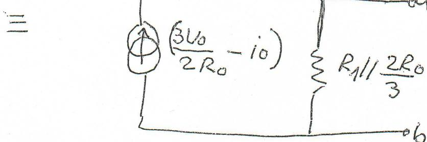
$$V_{ab} = \left( \frac{3V_0}{2R_o} - i_o \right) \cdot \left( R_1 / \frac{2R_o}{3} \right)$$
