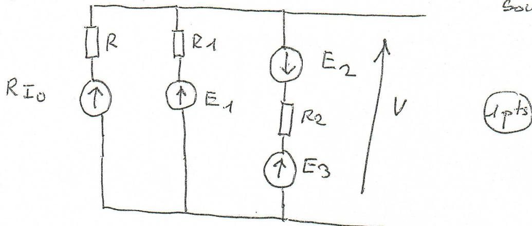
$$V = \frac{I_o + \frac{E_1}{R_1} + \frac{E_3 - E_2}{R_2}}{\frac{1}{R} + \frac{1}{R_1} + \frac{1}{R_2}}$$
