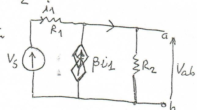
$$V_{Th} = V_{ab}$$
