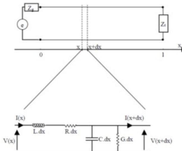
$$\text{On a } V(x, t) = Ldx \frac{\partial I(x, t)}{\partial t} + Rdx I(x, t) + V(x + dx, t)$$
