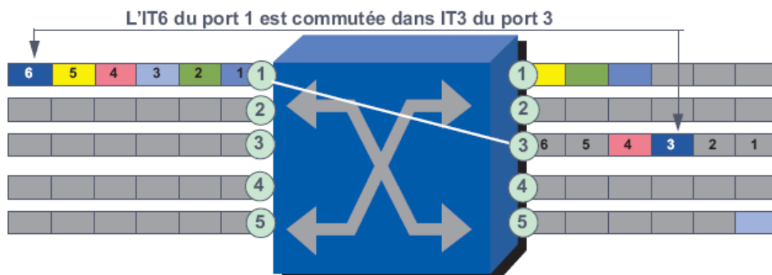
Figure III.11 – La commutation temporelle.
