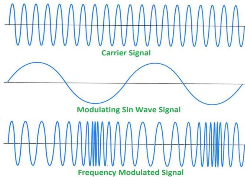
Figure.1. Modulation AM, PM et FM
