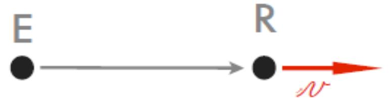
$$\mathcal{E}(f, t, \mathbf{u}(t)) = \frac{\alpha_s(\theta, \phi, f) \cos 2\pi f_0(t - r_0/c - vt/c)}{r_0 + vt}$$
