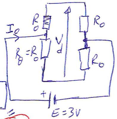
b/ le courant  $I_0$  :  $I_0 = \frac{E}{R_{eq}} = \frac{E}{2R_0 // 2R_0} = \frac{E}{R_0}$  (1)
