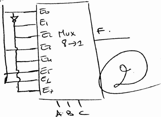
$$F = \bar{A}\bar{B}\bar{C} \cdot E_0 + \bar{A}\bar{B}C E_1 + \bar{A}B\bar{C} E_2 + \bar{A}B C E_3 + A\bar{B}\bar{C} E_4 + A\bar{B}C E_5 + AB\bar{C} E_6 + ABC E_7$$
