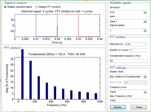
Figure.(3): diagramme de spectre, charge R
