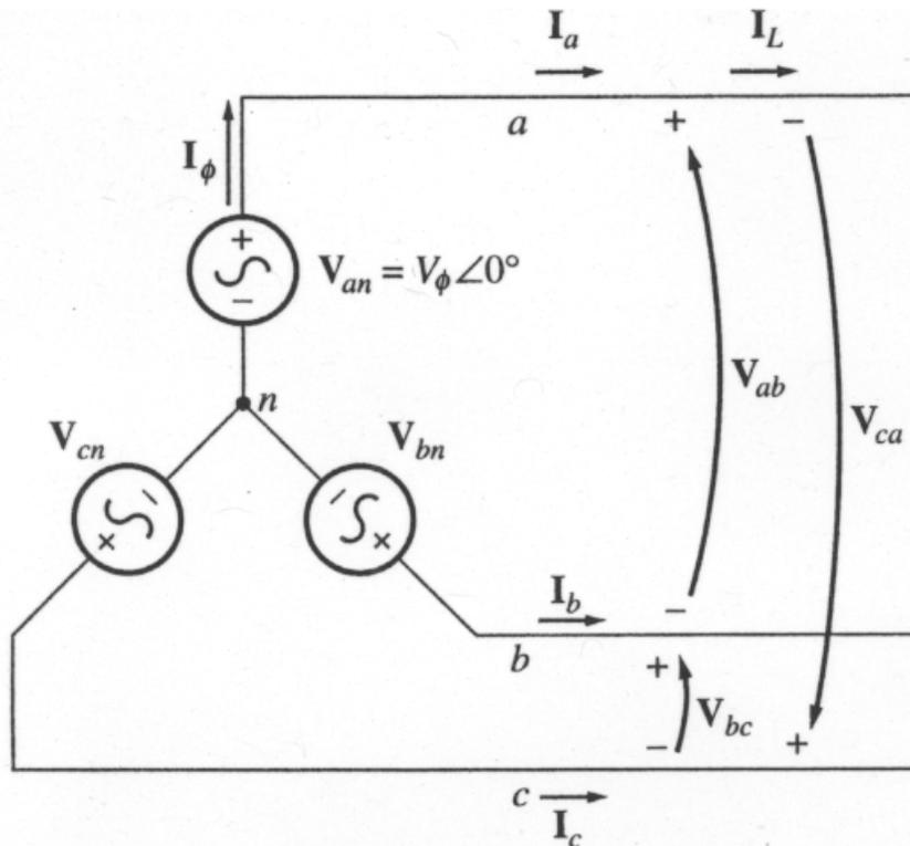
$$I_a = I_\phi \angle 0^\circ$$
