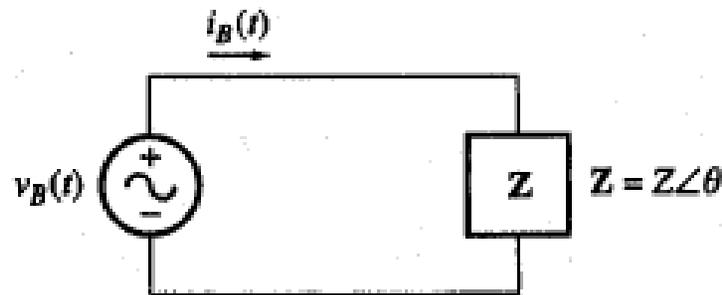
$$v_B(t) = \sqrt{2} V \sin (\omega t - 120^\circ) \text{ V}$$
