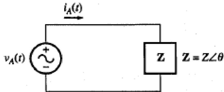
$$v_A(t) = \sqrt{2} V \sin \omega t \text{ V}$$
