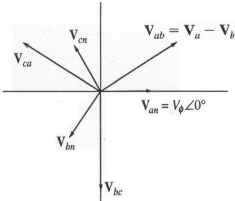
$$\begin{aligned} V_{ab} &= V_a - V_b \\ &= V_\phi \angle 0^\circ - V_\phi \angle -120^\circ \\ &= V_\phi - \left( -\frac{1}{2} V_\phi - j \frac{\sqrt{3}}{2} V_\phi \right) \\ &= \frac{3}{2} V_\phi + j \frac{\sqrt{3}}{2} V_\phi \\ &= \sqrt{3} V_\phi \left( \frac{\sqrt{3}}{2} + j \frac{1}{2} \right) \\ &= \sqrt{3} V_\phi \angle 30^\circ \end{aligned}$$
