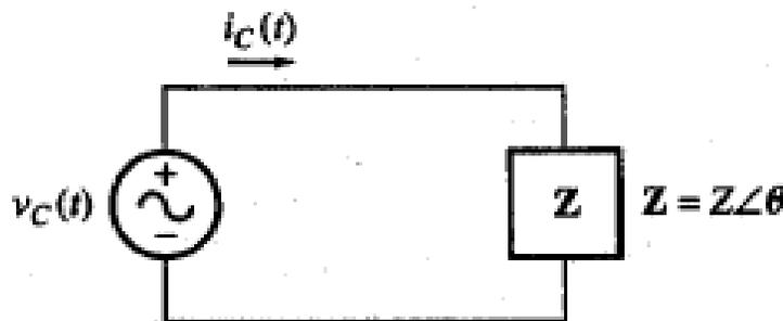
$$v_C(t) = \sqrt{2} V \sin (\omega t - 240^\circ) \text{ V}$$
