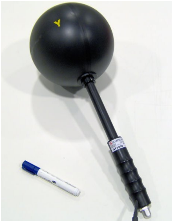
Isotropic antenna AT3000 (passive probe, 20 MHz – 3000 MHz)
